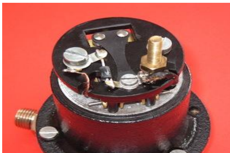
A typical TVS diode installation in an SU pump
