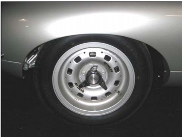
Lightweight Replica XK-E featured Dunlop racing wheels like the earlier D-types
