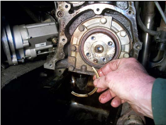
Rich found this missing thrust washer in the oil pan, just like Bob Canfield predicted.
