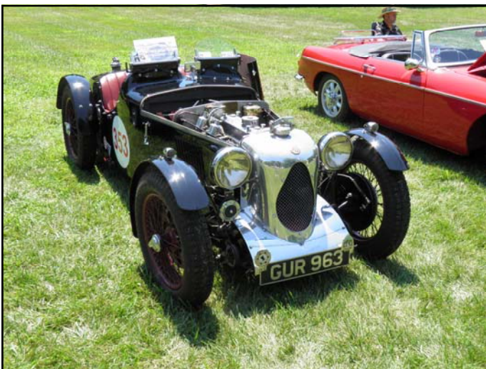
An MG P-series racer from 1935. The gearbox and bell housing sit, unguarded, right next to the driver's legs, ready to perform an instant amputation in the event of a mishap.
