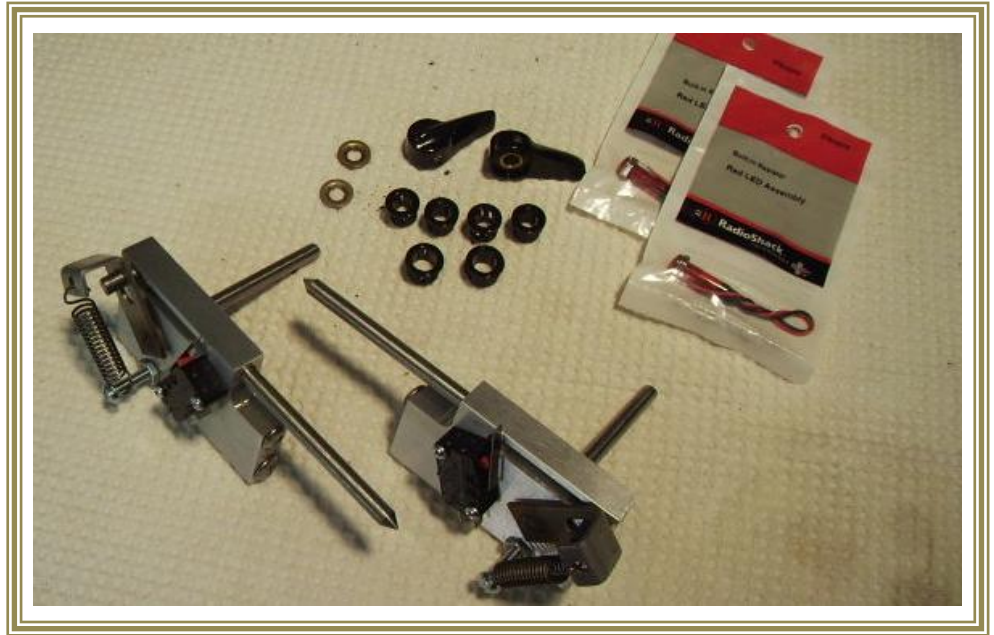
Above: The assembled parts, including the Carolina Custom Hot Rod Parts suicide door safety pin kit, Part No. SPD200, and the RadioShack indicator lights. Below: The pin, 2" longer than normal. Note: The pin is partially obscured by a mounting screw.
