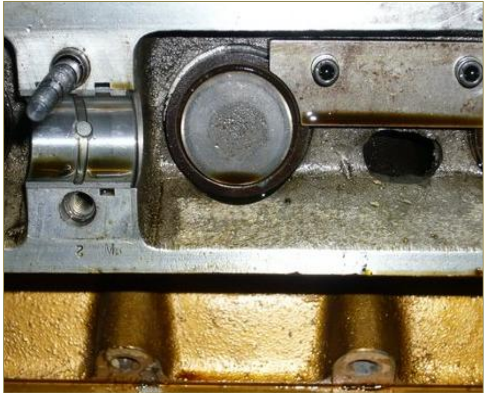
Above: An original tappet installed in the cylinder head. Note the heavy spalling on the tappet surface. Below: The underside of one of the intake valve tappets showing deposits due to blow-by of exhaust gases when the intake valve was closed. This indicates that the valve was not seating properly. Photos by Dick Nobile.
