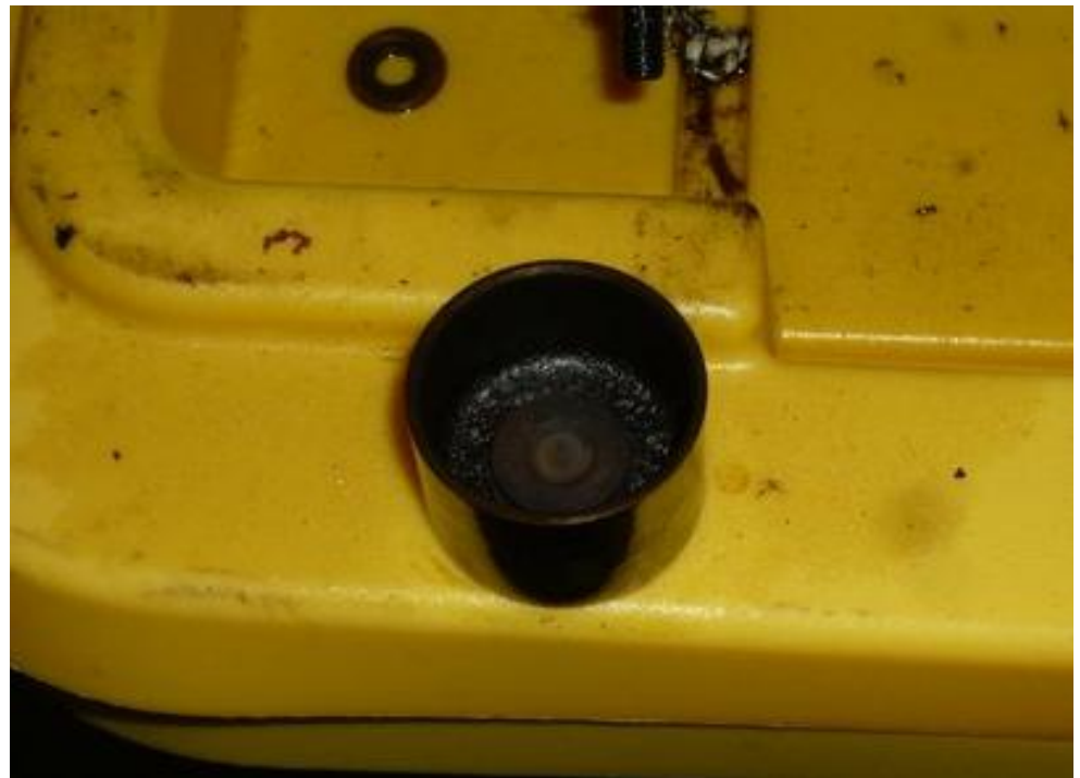
Above: An original tappet installed in the cylinder head. Note the heavy spalling on the tappet surface. Below: The underside of one of the intake valve tappets showing deposits due to blow-by of exhaust gases when the intake valve was closed. This indicates that the valve was not seating properly. Photos by Dick Nobile.
