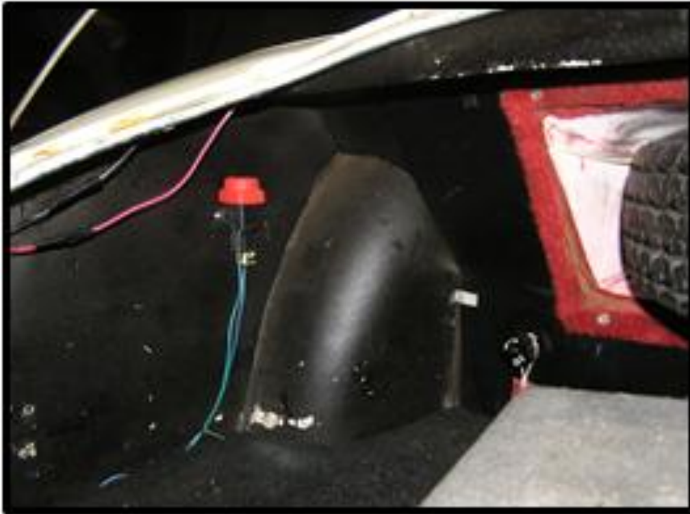
Fuel Pump Inertia Switch Installation (Moss Part Number 900-240)
