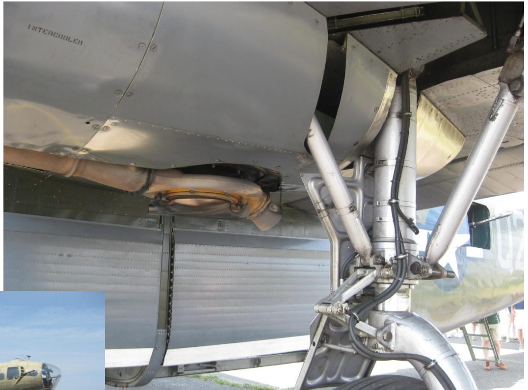
Above, left: Tail guns of the B-24 Liberator. Above: B-24 landing gear strut. Round object to the left is an engine turbocharger. Left: The legendary B-17 in all its glory.
