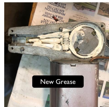
Before & after wiper-motor gearbox. Gearbox photos courtesy of Russ Sharples.
