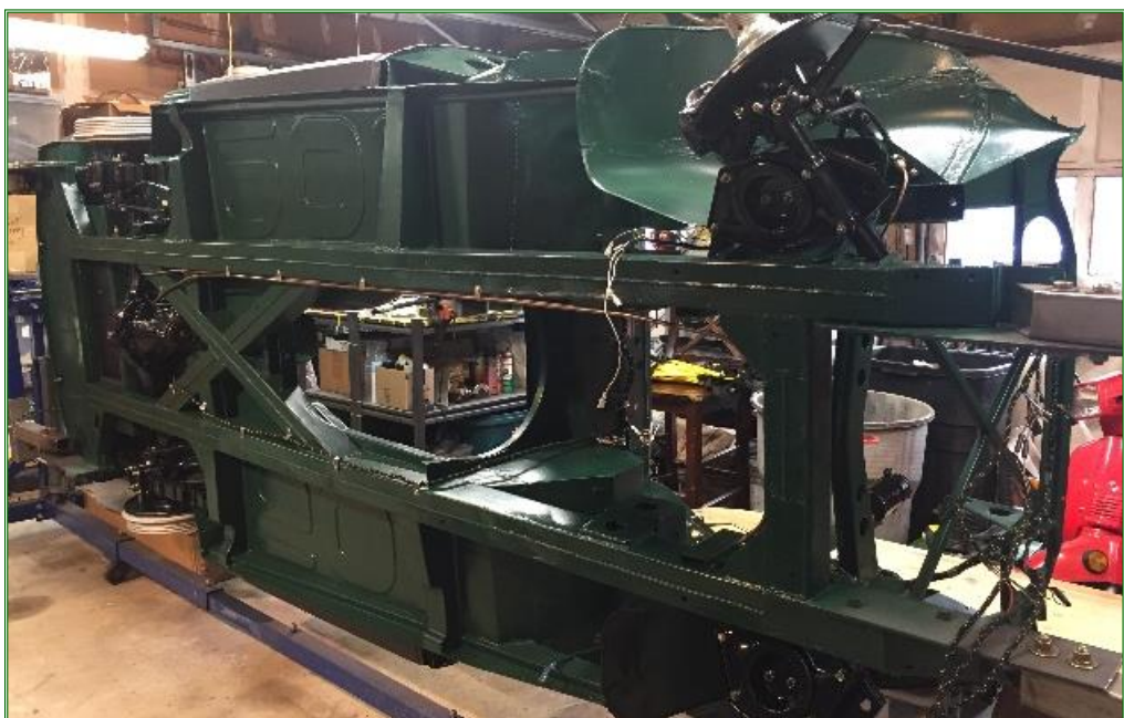
PHOTOS ON PAGE 1, ABOVE AND BELOW: Mike Kusch stands by while I start her up. The engine started for the first time under my ownership. It was seized when I bought the beautiful rust-bucket. The body prior to painting. PHOTOS ON THIS PAGE: My car rotisserie enabled me to turn the chassis a full 360°, making it easy to work on all sides of the car. Shown is the chassis, October 2020.
