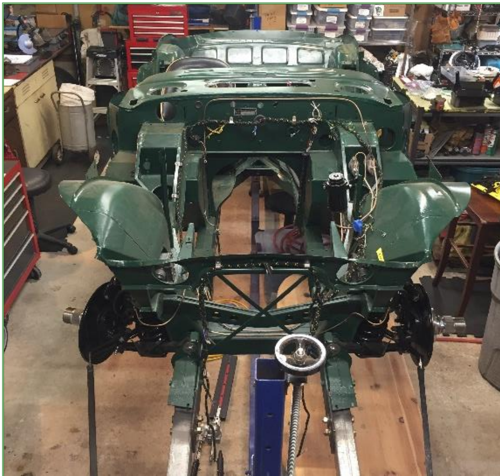
PHOTOS ON PAGE 1, ABOVE AND BELOW: Mike Kusch stands by while I start her up. The engine started for the first time under my ownership. It was seized when I bought the beautiful rust-bucket. The body prior to painting. PHOTOS ON THIS PAGE: My car rotisserie enabled me to turn the chassis a full 360°, making it easy to work on all sides of the car. Shown is the chassis, October 2020.
