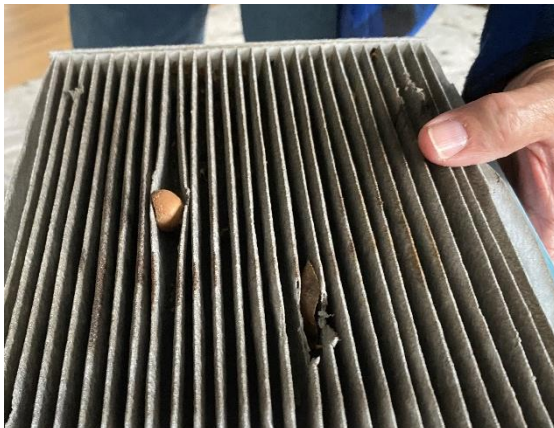
RIGHT: Cabin filter needing replacement. Photo by Rich Dalfonzo.
