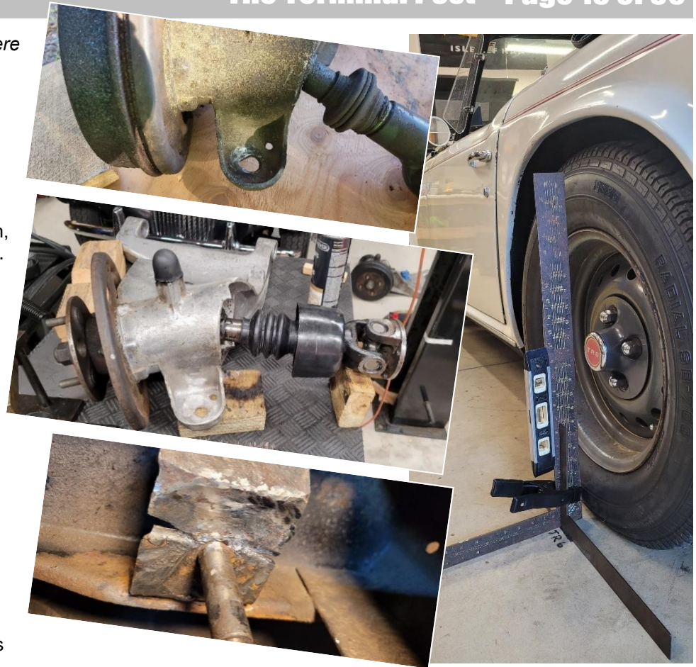
FROM TOP, LEFT: Half shaft and trailing arm, left side, before and after clean up. Broken differential mount prior to repair. TOP, RIGHT: Makeshift set up for camber measurement. Photos courtesy of Pete Dow. BOTTOM: Gathering around and under one of the lifts at Art Becker's son Wes's pole barn are, from left, Pete Dow, Tom Vash, John Quelch, Bob Canfield, and Jim Lamb. Taking a break, seated, is Bob Moser.
