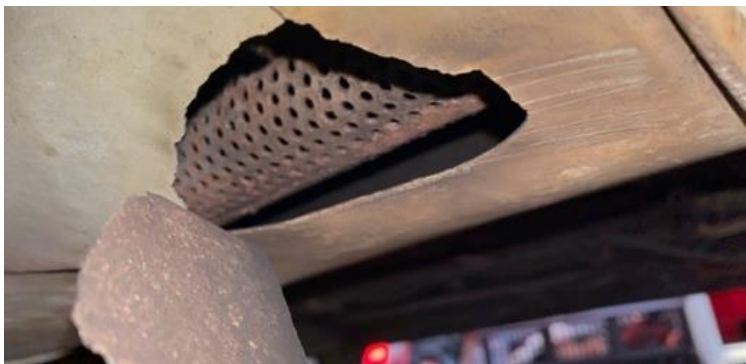
ABOVE: Cylinder head rebuilt by Bison Machine. BELOW: Huge hole blown in the muffler.
