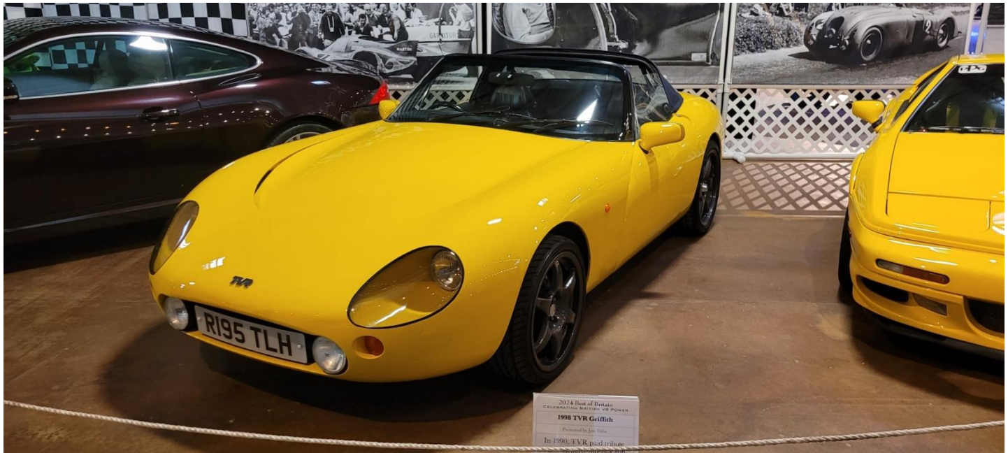
1990 TVR Griffith 500. weighing 2400 lbs., it is powered by 5-liter version of the Rover V8. This incredibly fast car was never officially imported into the US.
