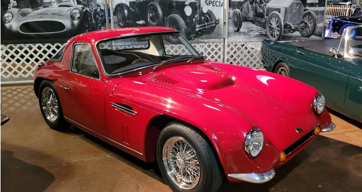
1967 TVR Tuscan V8 SWB. TVR combined a tube chassis, independent suspension, and a light fiberglass body, with a Ford V8 engine. This version is only one of 28 short wheelbase Tuscan V8s
