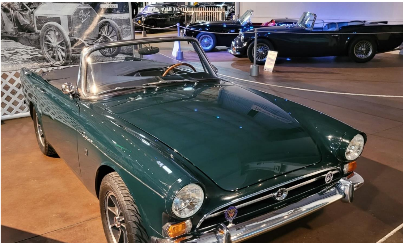
Another familiar car is this 1966 Sunbeam Tiger, Mk 1A. The Sunbeam Tiger replaced a heavy 4-cyl with a light V8, similar to the AC Cobra. This Tiger is one of approximately 2700 Mk 1A cars with the body and Trim found on the Series V Alpine.
